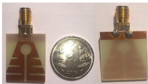
Figure 2: Prototype of the Conical Shaped Multiband Monopole Antenna (left: top view; right: bottom view).
